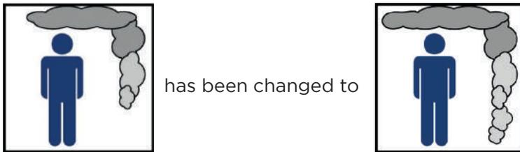
3. The smoke collects in a thicker layer near the ceiling, just above head height for an adult.
